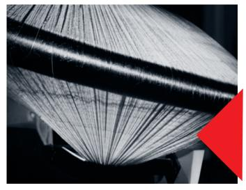
The production process involves a number of key stages – mixing of the raw materials, dissolving, filtering and finally spinning, when the fibre filaments are formed by forcing the processed cellulose through fine jets.
